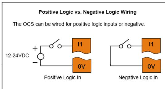
Digital inputs may be wired in either a Positive Logic or Negative Logic fashion as shown. The setting in the Cscape Hardware Configuration for the Digital Inputs must match the wiring used in order for the correct input states to be registered. No jumper settings are required for XLEe/XLTe. When used as a normal input and not for high speed functions, the state of the input is reflected in registers %I1 – %I12.
