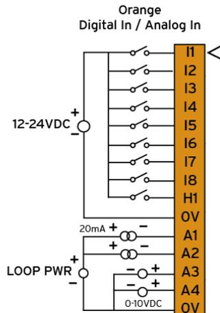
**NOTE:** The 0V terminals are internally connected.
