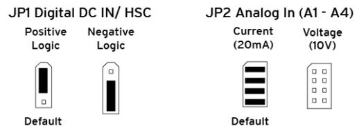
**NOTE:** The Cscape Module Configuration must match the selected I/O (JP) jumper settings.
