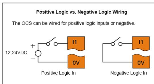
Digital inputs may be wired in either a Positive Logic or Negative Logic fashion as shown. The setting in the Cscape Hardware Configuration for the Digital Inputs must match the wiring used in order for the correct input states to be registered. When used as a normal input and not for high speed functions, the state of the input is reflected in registers %I1 – %I12.
