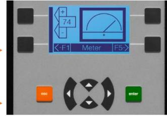
**Soft Keys**—The black squares on the sides of the screen are called “soft keys” and can be used to select objects that have an arrow icon pointing to the soft key. Soft keys can be assigned to certain objects, such as switch objects or jump objects.
