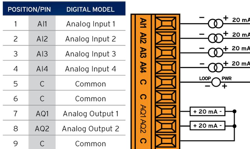
Figure 8.7 - Model R and A Analog In and Out
