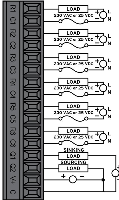
NOTE: Internal 10kΩ resistors between: V+ and Q1; V+ and Q2
