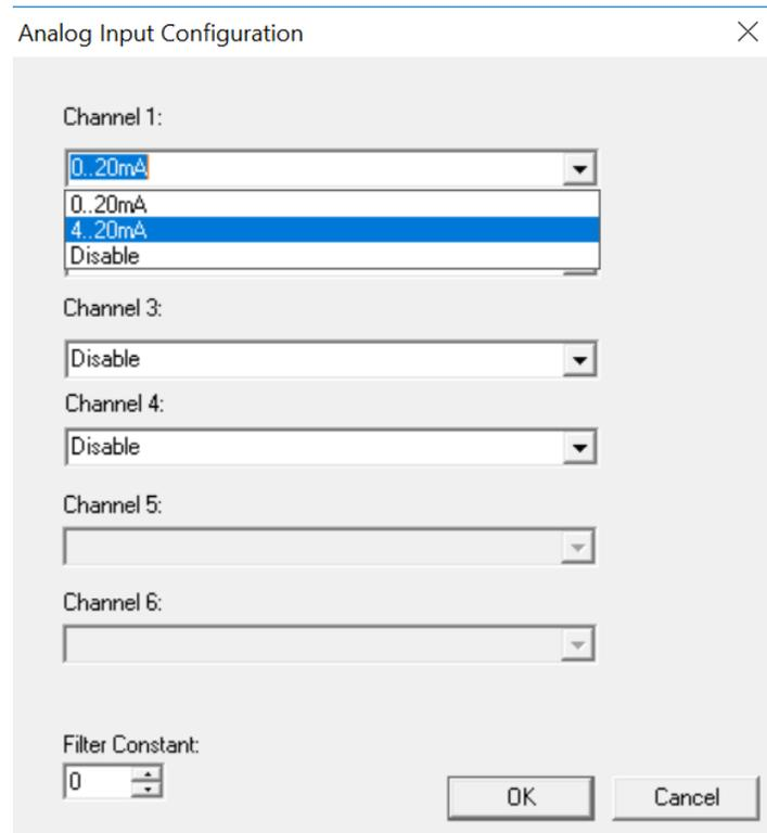
Figure 7.10- Analog Input Configuration Dialog
