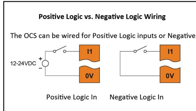
Figure 8.5 - Positive and Negative Inputs
