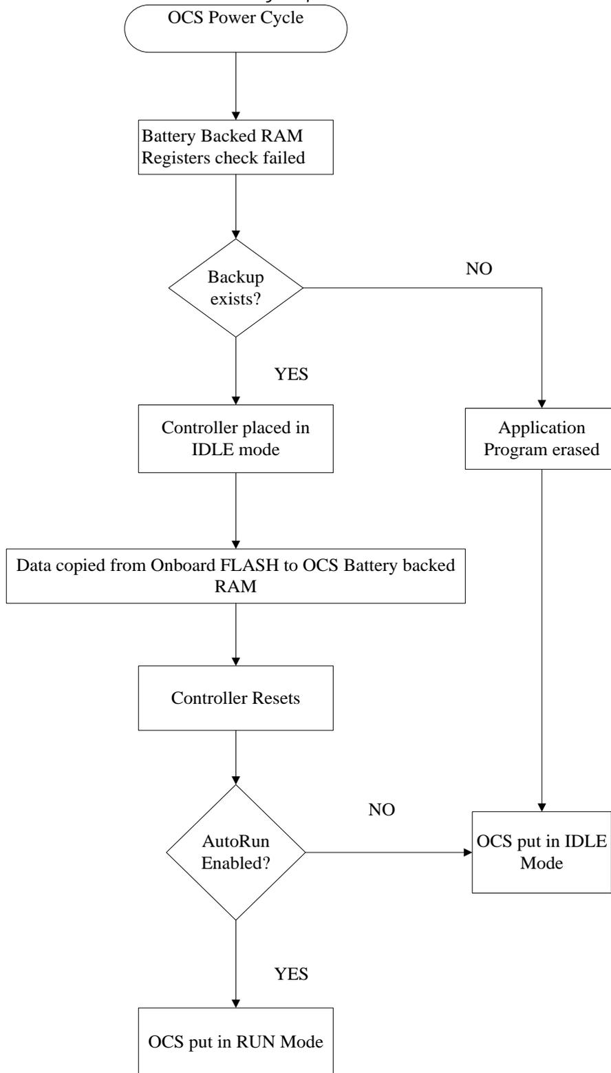
Figure 16.5 - Flow Chart for Automatic Restore
