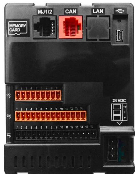
Figure 11.1 - CAN Connector (Red)
