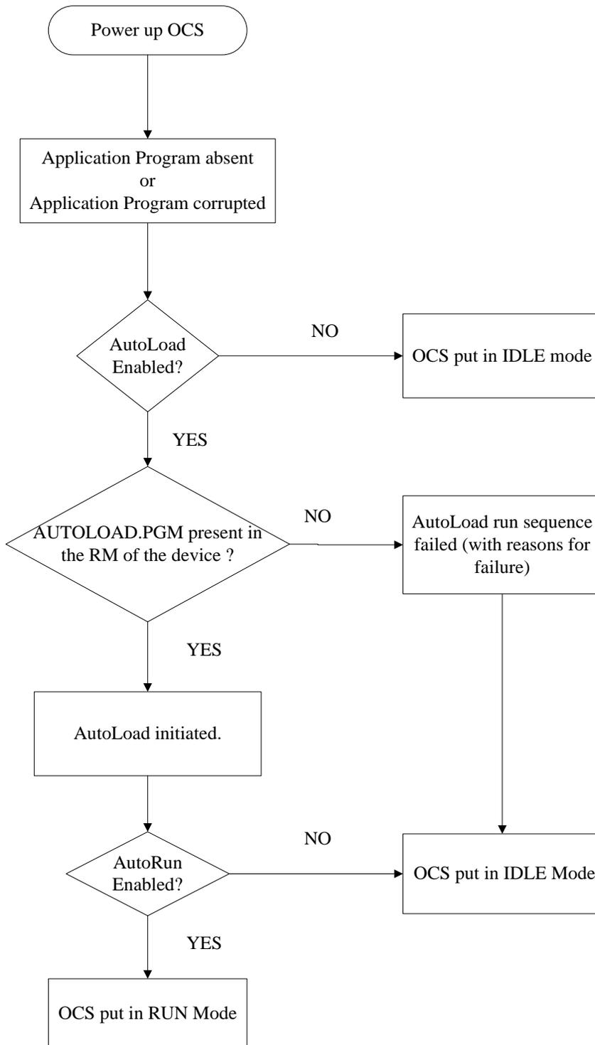
Figure 16.7 - Flow Chart for AutoLoad
