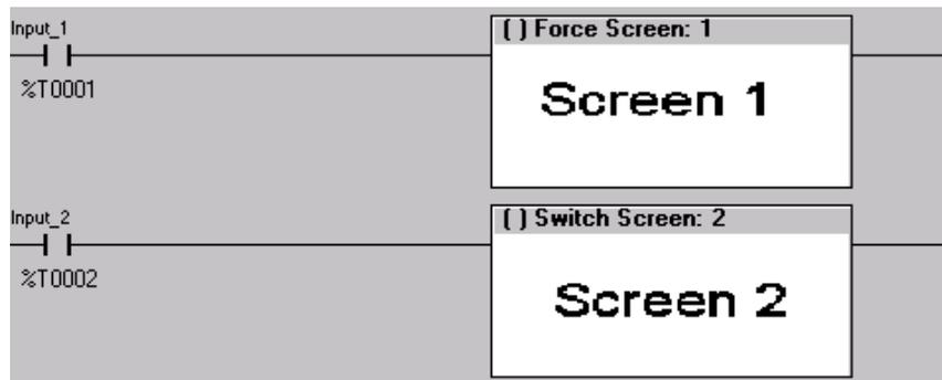
Figure 12.4 - Force and Switch Coils in Ladder Programming
