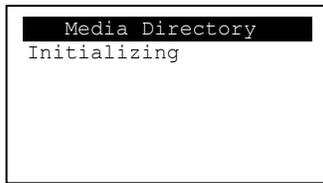
= Micro SD card is installed, but it is still initializing
