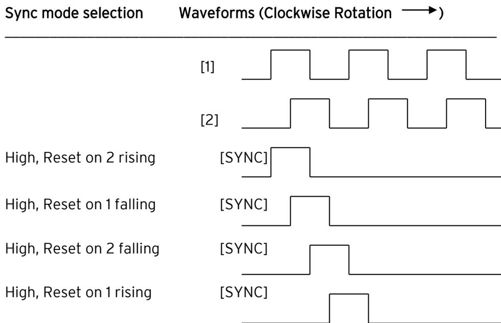
\*While not displayed in this figure, modes for low level (inverse logic) are also supported for each state.
