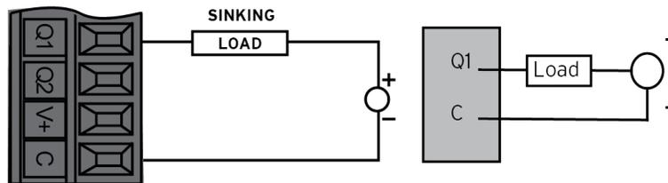
**Sinking:** Outputs can sink 500mA
