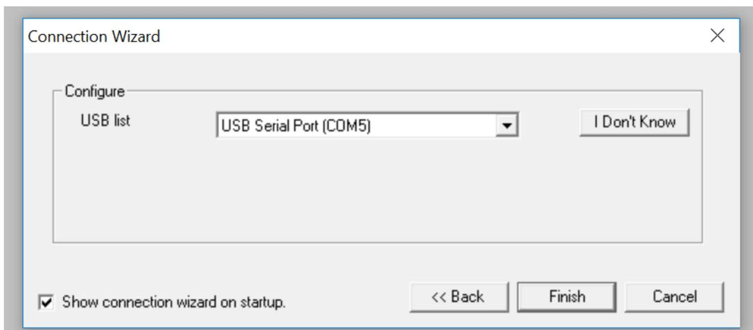
If the Connection Wizard does not pop up upon opening Cscape, then select **Controller** (in the Cscape tool bar) → **Connection Wizard**, choose your connection method. If you are connecting for the first time, we suggest connecting via USB.
