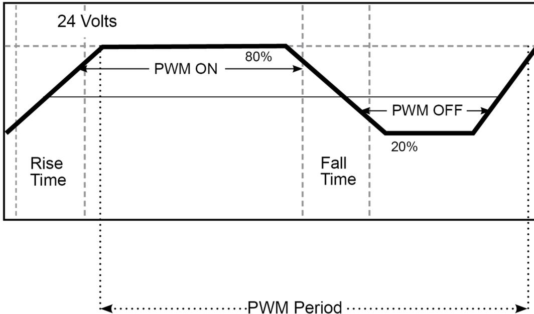
Figure 9.2 - PWM Output Waveform
