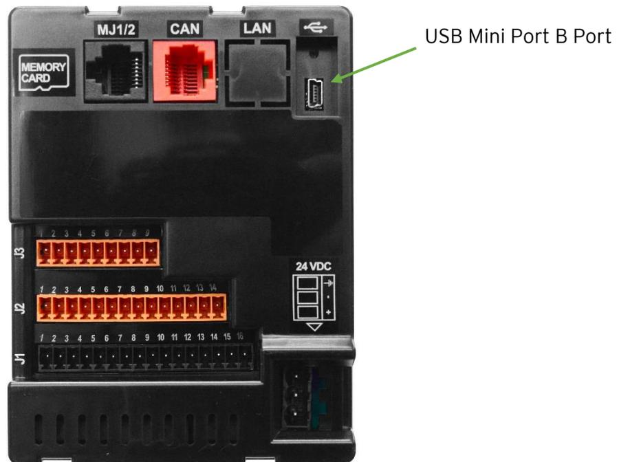
Figure 7.2 - USB Programming Connector
