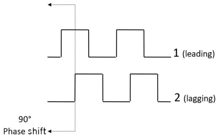
Using the above waveforms and an HSC input configuration of "Quadrature" - "1 leads 2, count up," the accumulator will count up when 1 is rising and 2 is low, 1 is high and 2 is rising, 1 is falling and 2 is high, and when 1 is low and 2 is falling. This results in 4 counts per revolution. In order to determine the number of cycles, the accumulator would have to be divided by 4.
