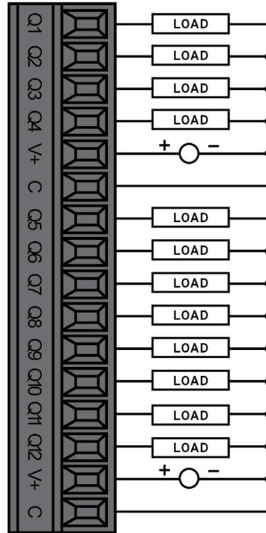
Figure 8.2 - Model A Digital Output
