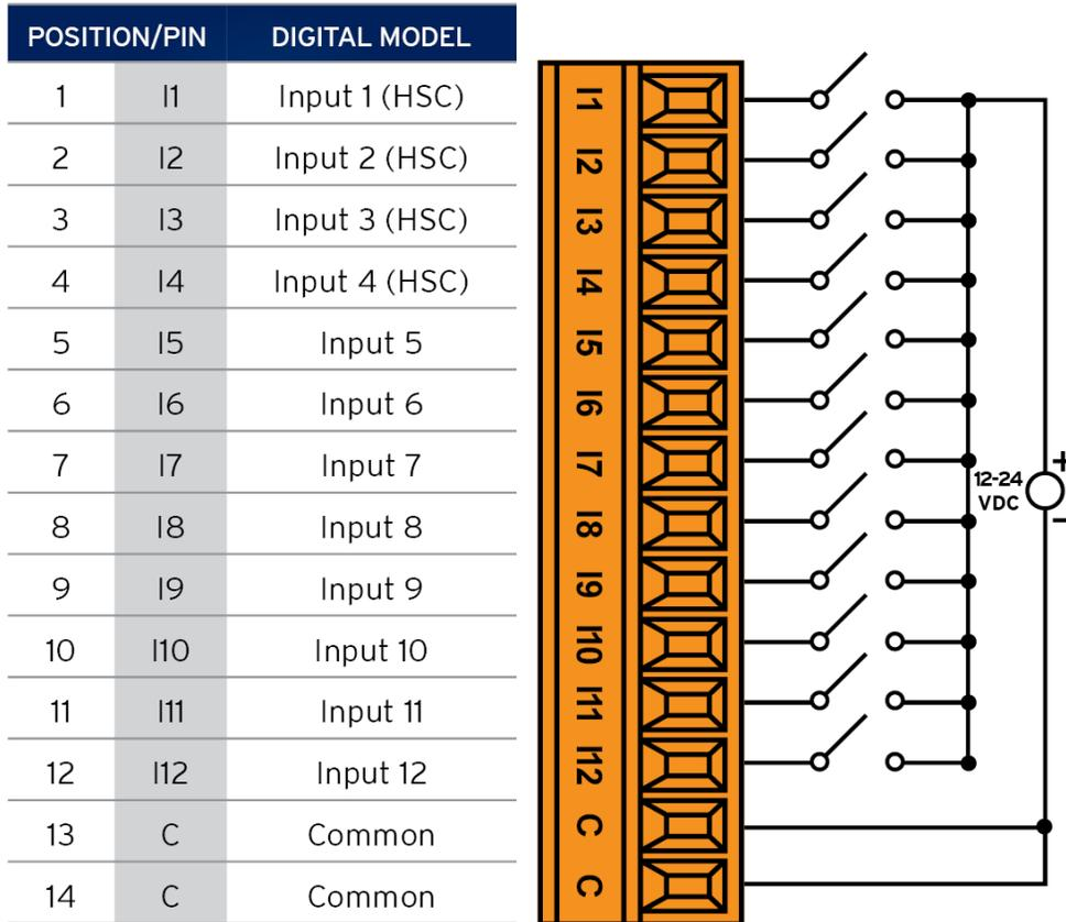
Figure 8.6 - Model R and A Digital Input
