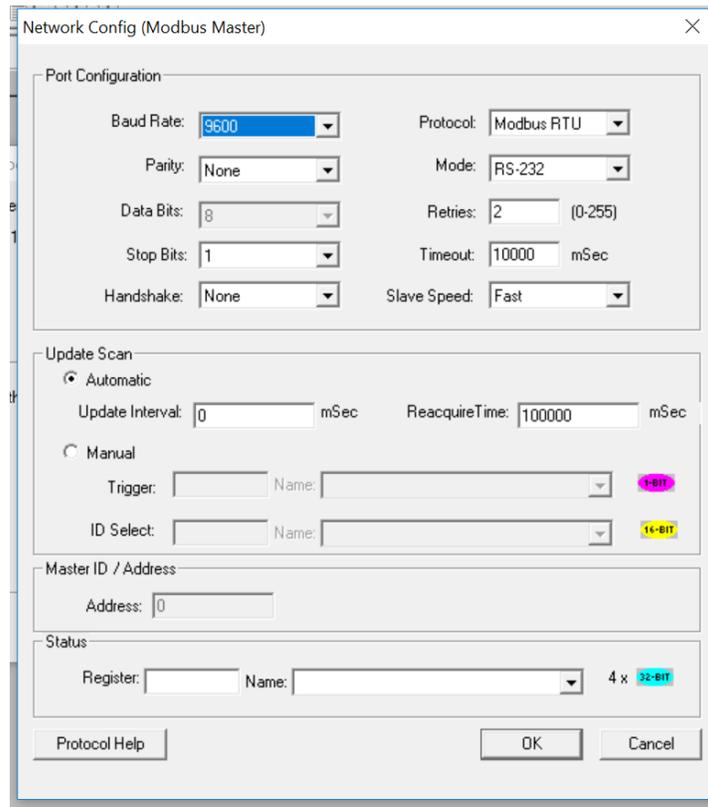
Network Configuration provides the required parameters to configure the network. Each protocol is different and may not require all the Network Config field. Please refer to the table below for the options in the Network Config field.
