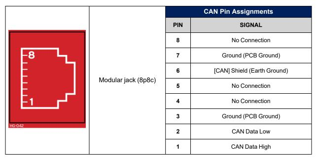
The CAN port is provided via the single 8-position modular jack labeled "CAN". It may be used to communicate with other OCS products using Horner's CsCAN protocol. Additionally, remote expansion I/O such as SmartRail, SmartBlock, and SmartStix may be implemented using the CsCAN protocol.
