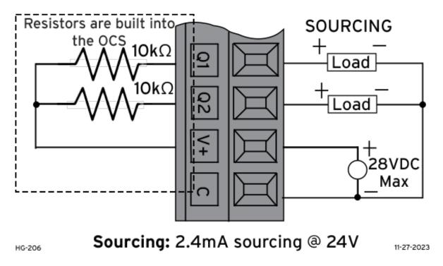
**NOTE:** Cscape offers a choice to flip the output by selecting "sourcing" as the output mode. This can come in handy when working with certain devices in this setup. It's important to note that this option doesn't alter the kind of output.
