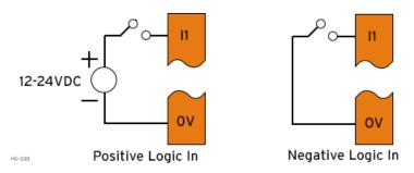
Digital inputs may be wired in either a Positive Logic or Negative Logic fashion as shown. The setting in the Cscape Hardware Configuration for the Digital Inputs must match the wiring used in order for the correct input states to be registered.
