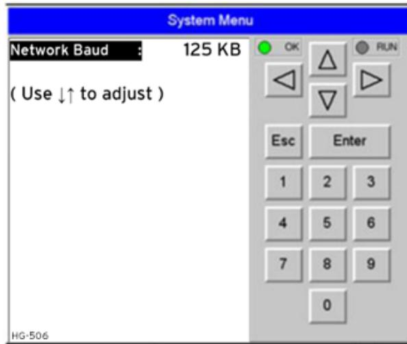
The Set Network Baud submenu for both X7 models displays just one System Setting and it is editable.
