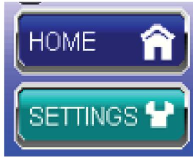
Screen jumps can also be triggered on other keys or based on control logic for more advanced applications. To allow the operator to change screens, a **screen jump object** is generally used. This object may be visually **represented as a button** (responding to touch) or remain invisible and logically tied to an OCS register. An optional system ICON may be configured for display along with the legend, which aids in identifying the object as one that causes a screen change.
