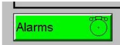
**Alarm Viewer** - To view, acknowledge and/or clear alarms, the operator must access the alarm viewer. This is accomplished by touching an (enabled) alarm object. When accessed, the alarm viewer is displayed as pop-up alarm viewer dialog similar to that shown below.
