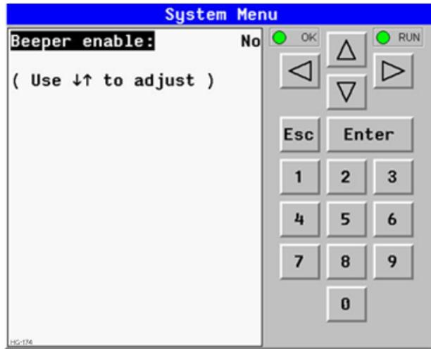
The Set Beeper submenu displays one System Setting, which is editable.
