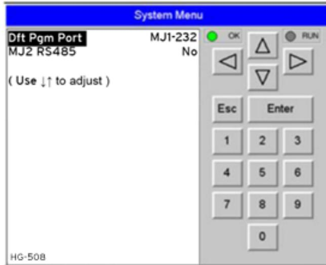
The Set Serial Ports submenu displays three System Settings, all of which are editable, and one optional item.
