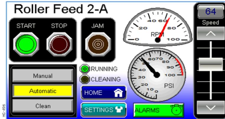
Multiple objects are provided for displaying data such as virtual panel lights, push buttons, numeric value displays, bar graphs, meters, graphs, and animated bitmaps. On the X7, these graphical objects (through ladder manipulation of attribute bits) can change color, flash, or change visibility to attract operator attention.
