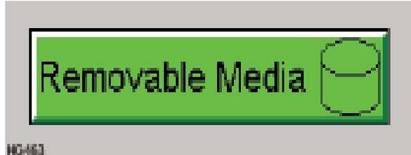
To view and perform file operations, the operator must access the removable viewer. This is accomplished by either touching an (enabled) removable media object or through the system menu. When accessed, the removable media viewer is displayed as pop-up removable media dialog similar to that shown in the figure below.
