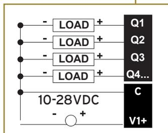
Digital outputs are Positive Logic. If an output is turned on, the voltage supplied at the QV+ terminal is applied to that output. When used as normal inputs, the state of the output may be controlled using the registers %Q1 - %Q10.
