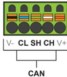
The CAN port is provided via three connections on the CAN/Power: CAN\_LOW (CL), CAN\_HIGH (CH), and V- (C). It may be used to communicate with other OCS products using Horner's CsCAN protocol.
