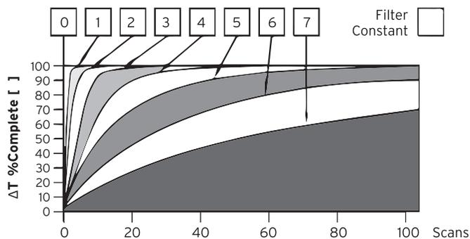
Digital filtering module response to a temperature change in the analog in. The illustration above demonstrates the effect of digital filtering on (set with Filter Constant).
