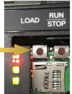
Two recessed buttons provide control of several RCC modes. The door may be opened to access the buttons.
