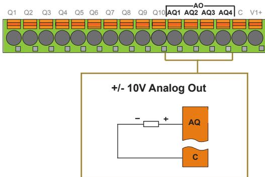
Each Analog Output may be specified for a range of -10VDC to +10VDC. The Analog Output registers %AQ1 - %AQ4 may be used to control the output by placing a value between -32000 to +32000 into the register. This may be directly from a PID loop output, for example.
