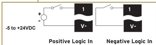
Digital inputs may be wired in either a Positive Logic or Negative Logic fashion as shown. The setting in the Cscape Hardware Configuration for the Digital Inputs must match the wiring used in order for the correct input states to be registered. The state of the inputs are reflected in registers %I1 through %I12. The Common connections are found on the top connector. Inputs 1-8 have programmable input voltage ranges and input frequency filters.
