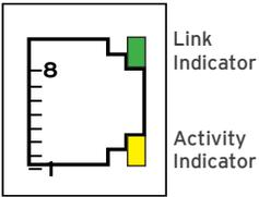
A 10/100 Ethernet port with automatic MDI-X (crossover detection) is provided via the single 8-position modular jack labeled "LAN". Several features are available for use over Ethernet, such as CsCAN, Modbus, TCP, Ethernet IP, and EGD.
