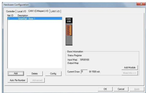
8. Now up to 8 modules can be added via the "Add Module" button. As I/O modules are added the Input Map, Output Map, and Current Draw are updated, showing the accumulated I/O Module Information. More details regarding each module can be viewed via the "More Info" button.
