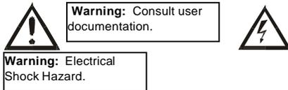
**WARNING: To avoid the risk of electric shock or burns, always connect the safety (or earth) ground before making any other connections.**
