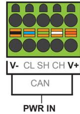
A single 5-pin connector is used to make both a network connection and power input. A quality Class 2 power supply should be used for this product. If the power is run with the network cable, care must be taken so that the voltage does not drop below the lower supply limit on longer runs.
