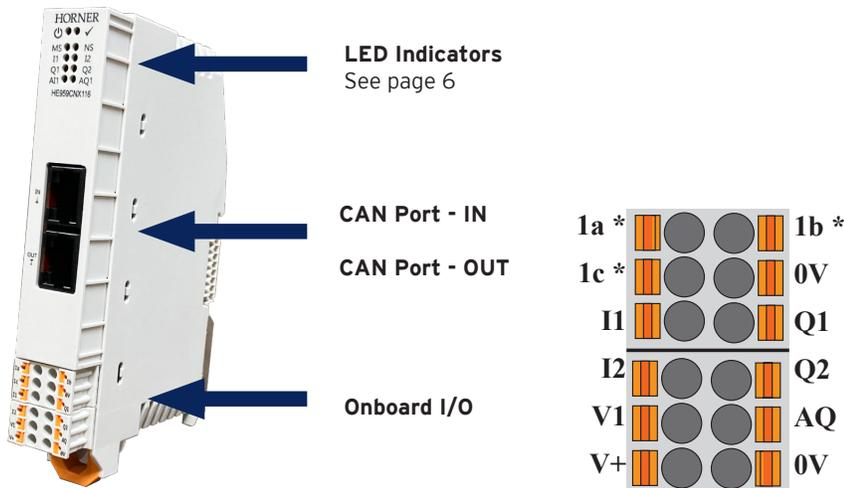
**\*WARNING:** Do not put voltage on 1a and no more than 12V on 1b or 1c ports. Doing so will damage the board.
