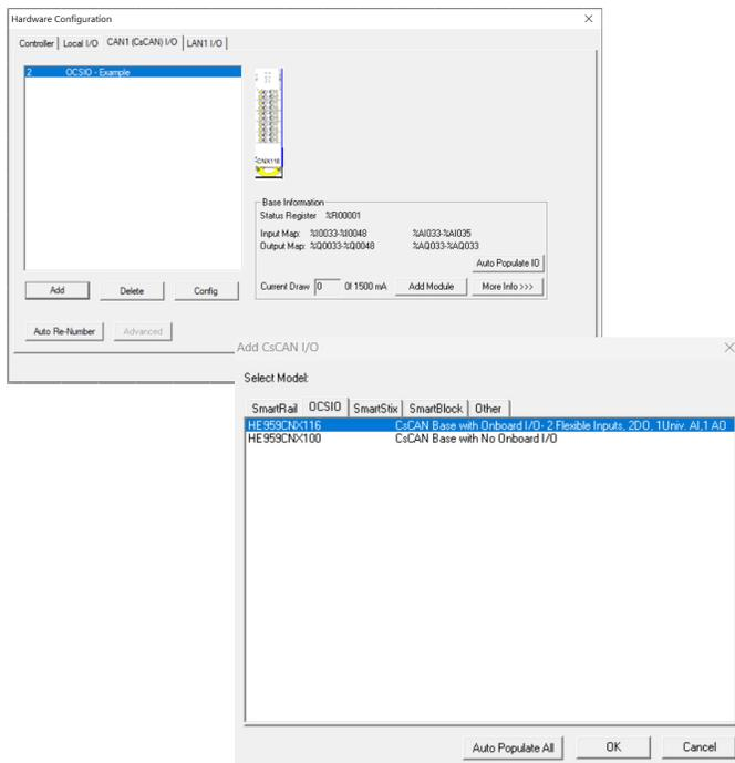
8. Now modules can be added via the "Add Module" button. As I/O modules are added the Input Map, Output Map, and Current Draw are updated, showing the accumulated I/O Module Information. More details regarding each module can be viewed via the "More Info" button.
